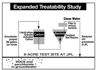
NASA plans to pump the groundwater and pipe it to a treatment facility to remove VOCs and perchlorate. The filtered treated water would then be reinjected into the groundwater beneath JPL.
