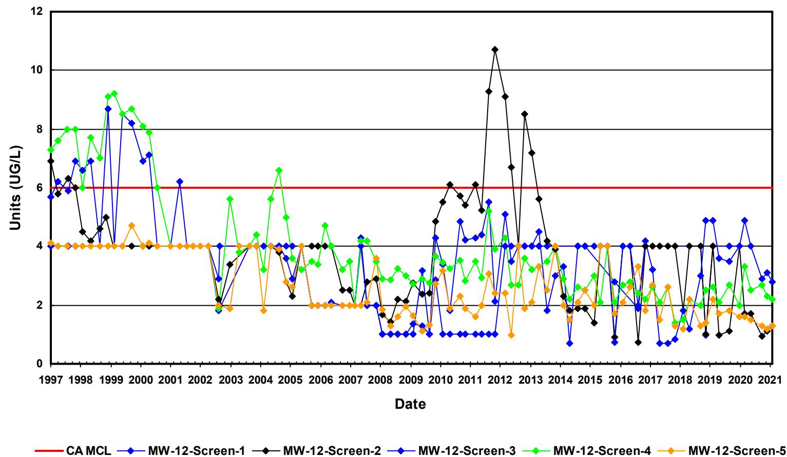
Reg Limit Type: CA MCL Parameter Name: Perchlorate Reg Limit: 6 Units: UG/L
