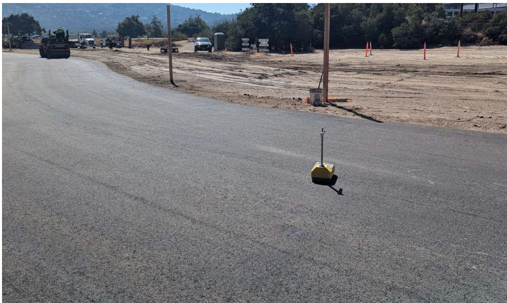
Image 1: Taking nuke gauge density reading on Asphalt layer at test location #6.
