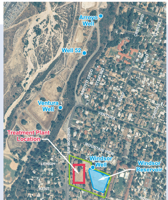
Four wells in Pasadena from which groundwater will be pumped to the new Monk Hill Groundwater Treatment Plant.
